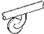
-25 Underslung Welded Support
